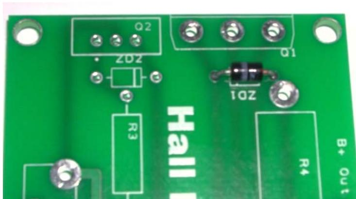
Step 3) Install the 10 ohm 5 watt resistor in the R4 location on the board.
