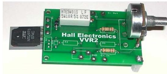
That completes the board assembly for a Cathode Biased Amp.
