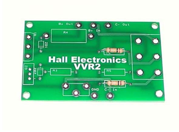
Step2) Install the 12v Zener diode at location ZD1 making sure the banded side of the diode is orientated like the image on the board
