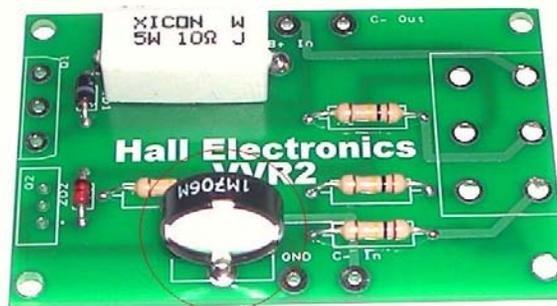
Step 9) Install the FET Q2. The FET is installed with the tab side towards the edge of the board. The mosfet is a static sensitive device. That means that static electricity that builds up in your body can blow the mosfet. Always make sure you use normal static precautions when handling the mosfet.
