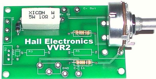
Step 5) Mount the mosfet on the board. The mosfet is a static sensitive device. That means that static electricity that builds up in your body can blow the mosfet. Always make sure you use normal static precautions when handling the mosfet. It can be mounted either on top of the board or on the bottom of the board.
